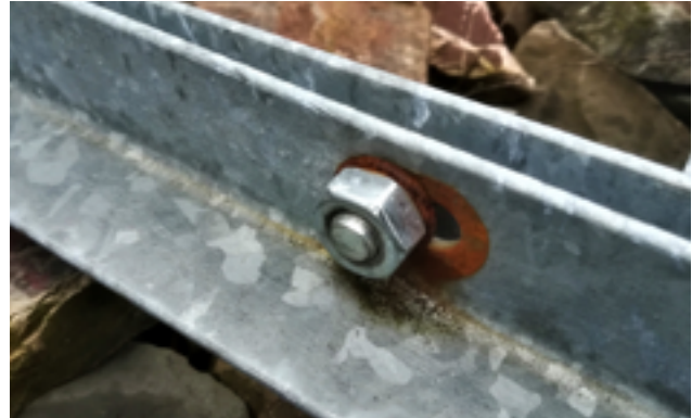
A galvanised washer and a stainless steel nut have caused a poor surface ratio (source: OBO Bettermann)
