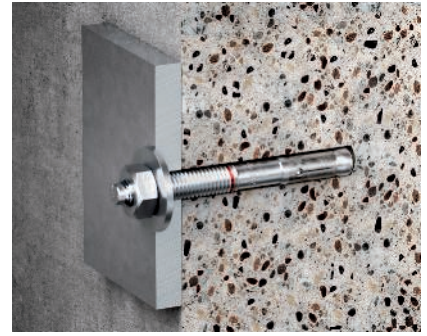
Bolt tie, type BZ Bolt tie, type BZ, for fastening heavy-duty anchorings in cracked or non-cracked standard concrete C20/25 to C50/60, suitable for push-through mounting, with M8, M10, M12 or M16 thread.
