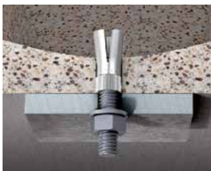
Hollow core anchor, type Easy Hollow core anchor, type Easy, with M6, M8, M10 and M12 internal thread, for use in stressed concrete core slab ceilings.
