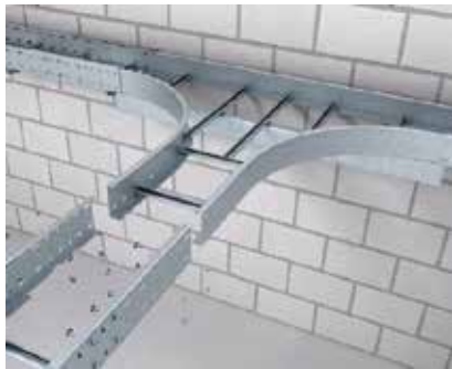
Mounting of tee Tee in combination with wide span cable ladder. The tee is connected to the wide span cable ladder using external connectors.
