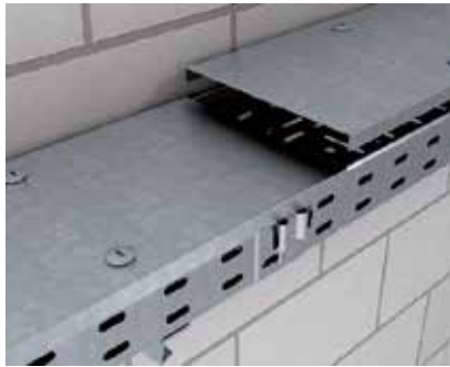
Cover mounting with turn buckle The cover is fastened to the cable tray using turn buckles; this is done by clamping the turn buckle under the rolled up side rail of the cable tray with a 90° turn.
