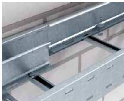
Screwed barrier strip fastening Barrier strip mounting in wide span cable ladders. Fastening using slide nuts and hexagonal bolts.
