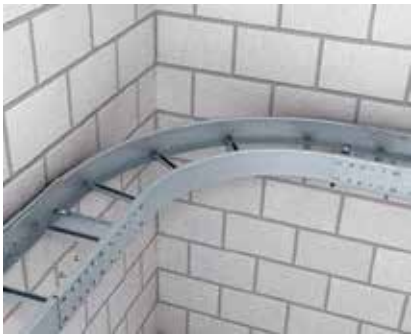
Mounting of 90° bend Bend in combination with wide span cable ladder. The bend is connected to the wide span cable ladder using external connectors.
