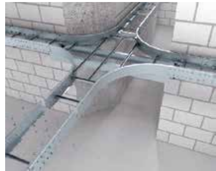
Cross-over mounting Cross-over in combination with wide span cable ladder. The cross-over is connected to the wide span cable ladder using external connectors.
