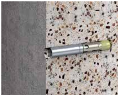
Bolt tie, type BZ-IG The bolt tie BZ-IG with internal thread is approved for normal drill holes which are not undercut. Within the scope of the European Technical Assessment ETA-99/0010 for cracked and non-cracked concrete, a system comprising nut and washer and a standard threaded rod can be used, as well as hexagonal bolts and countersunk head screws.
