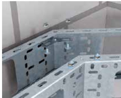
Angle connection Simple bend creation with hinge connectors, type SV. For this, the side rails must be cut.
