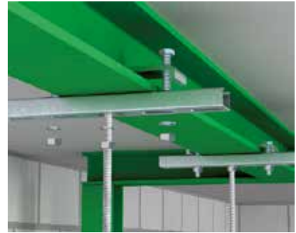
Steel clamping, C profile rail Fastening of a C profile, type MS 4022 or MS 5030, to steel girder using clamping angles, type KWS.
