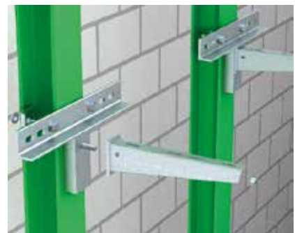
Clamp fastening on vertical steel girder Mounting of the adapter plate, type KA-AW, on the vertical steel girder using clamping angles or chuck jaws. Wall brackets of type AW are fastened to the adapter plate, using the hexagon head screw, type SKS 12x40 GF.
