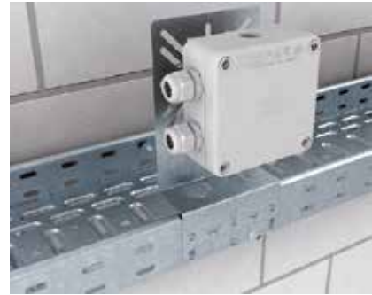
Mounting plate with quick fastening Fastening of the mounting plate, type MP, on the side rail of the cable tray. The mounting plate can be fastened to the rail with quick connectors, and permanently fastened using truss-head bolts of type FRSB 6x12 mm.
