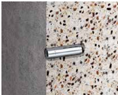
Impact tie, type ES Impact tie, type E, with M6, M8, M10, M12 internal thread. To accept small loads, approved for multiple fixings in cracked and non-cracked concrete of non-load-bearing systems.
