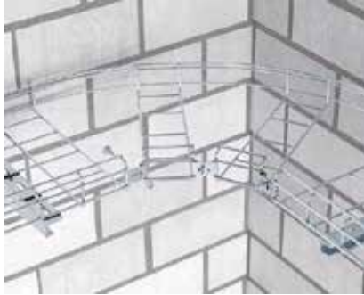
Horizontal bends Implementation of a horizontal bend for C mesh cable trays with corner connector, type GEV 36.
