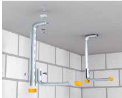
Mounting of TP suspended support with single-sided bracket fastening Ceiling mounting of a TP suspended support with spacer DS 4 and one-sided bracket mounting. Maximum tray width 300 mm.
